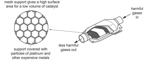
Suggest the advantages of using a low volume of catalyst with a high surface area.
