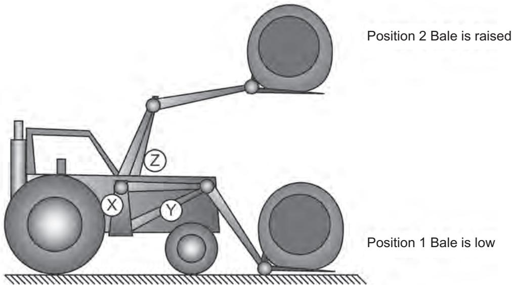
X is the position of the tractor's centre of gravity when it is not carrying any bale.
