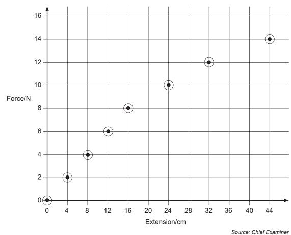
(i) Draw a line through all the points and use it to estimate the force that corresponds to the limit of proportionality for the spring.
