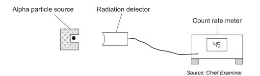
The distance between the alpha source and the radiation detector is changed. The reading on the count rate meter is noted in counts per second (cps) for each distance.
