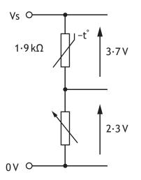
Calculate the resistance of the variable resistor for these conditions.
