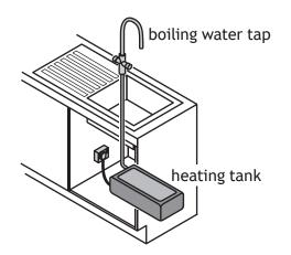
Water is boiled in the heating tank and then stored until it is ready to be used. 1.4 MJ of electrical energy is used when heating a full tank of water for the first time.
