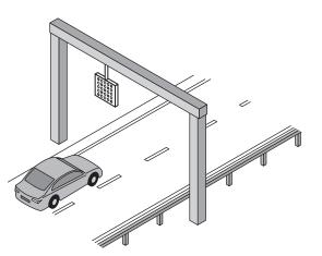
The sign produces a downward force of  $5 \cdot 2 \text{ kN}$  and the weight of the gantry itself is 22 kN.
