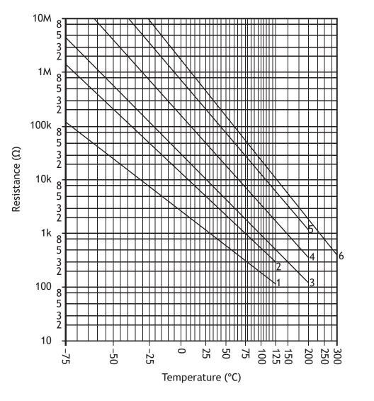
Determine, with reference to this graph, the resistance of the type 1 thermistor at 40  $^{\circ}$ C.
