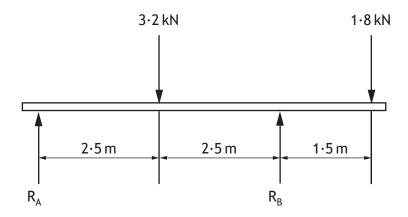
(a) (i) Calculate the size of reaction force  $R_A$ , by taking moments about  $R_B$ .
