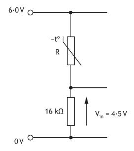
(b) Calculate the resistance R, when  $V_{in} = 4.5 V$ .
