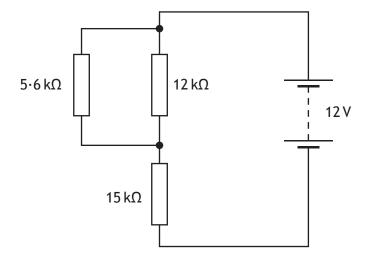
(b) Calculate the total resistance of this circuit.
