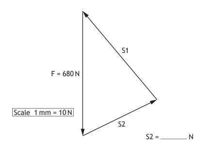
(d) A maximum of two acrobats can hang from the trapeze swing at any one time. When this happens the forces in support wires S1 and S2 are as follows:
