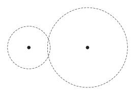
Describe two errors that were made when drawing this simple gear train.
