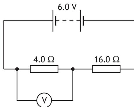
Calculate the reading on the voltmeter.
