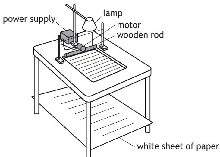
The wooden rod moves in and out of the water to generate water waves.
