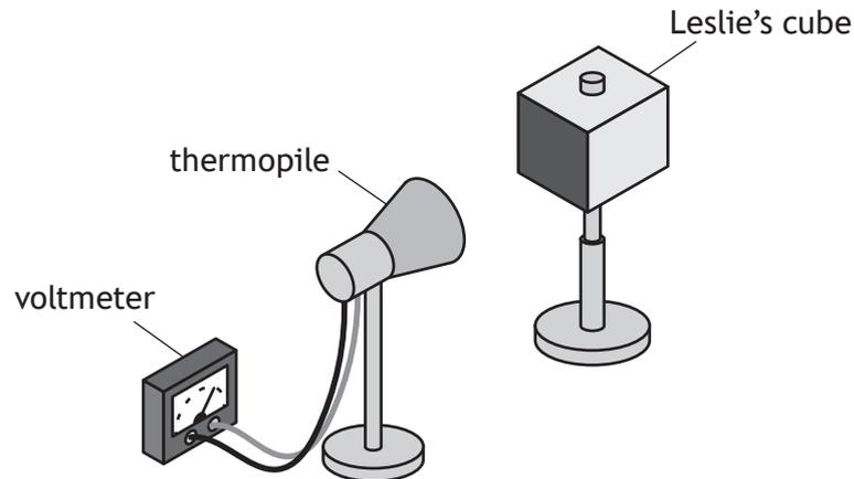
The student fills the cube with hot water and measures the amount of infrared radiation at different distances from the cube, using the thermopile.
