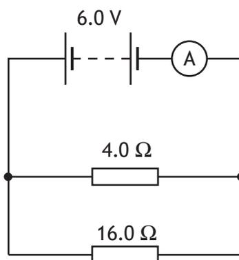
(i) Calculate the total resistance of the circuit.
