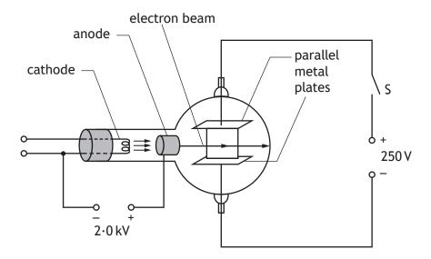
(a) Electrons are accelerated from rest between the cathode and the anode by a potential difference of  $2.0\,\mathrm{kV}$ .
