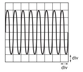
The timebase control of the oscilloscope is set at 2 ms/div.
