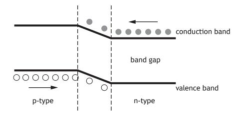
(i) A voltage is applied across an LED so that it is forward biased and emits light.
