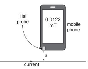
He varies the distance, *a*, from the wire to the edge of the phone and measures the magnetic flux density each time. The current is kept constant. His results are shown in the table.
